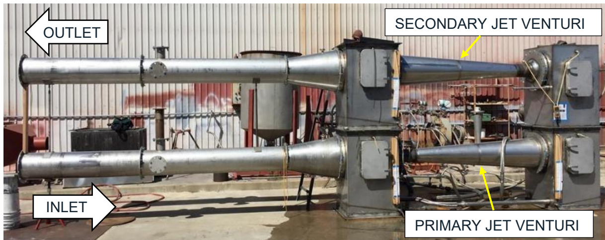
Figure 4: A two-stage Jet Venturi Scrubber pilot unit.
